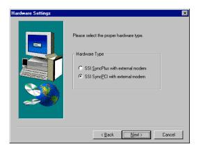
? If you are using the SSI SyncPlus, select the IRQ and I/O port address setting. During installation you should make choices that match the settings on the adapter and do not conflict with other hardware in your machine.
